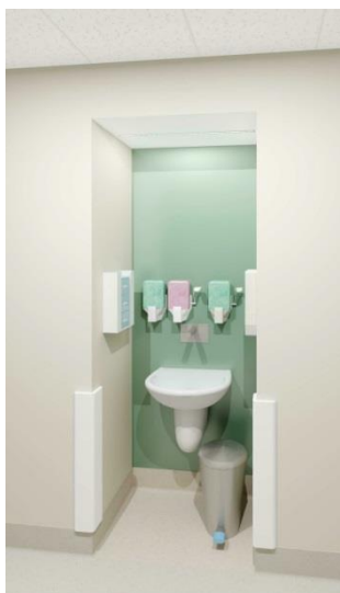
Figure 2.9: Reduced height ceiling within a corridor bay
