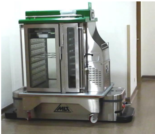
Figure15: Typical AGV with a supply trolley
